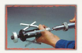
Orbiter I coats 3.5-inch through 7-inch pipes.
