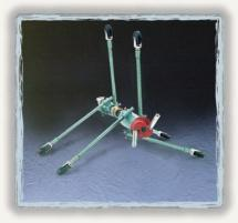
In operation, two standard nozzles installed on the head cause the head to rotate and propel abrasive to the pipe surface for incomparable hitting force. SB-3660 uses long venturi nozzles for effective blasting of larger ID pipe.
